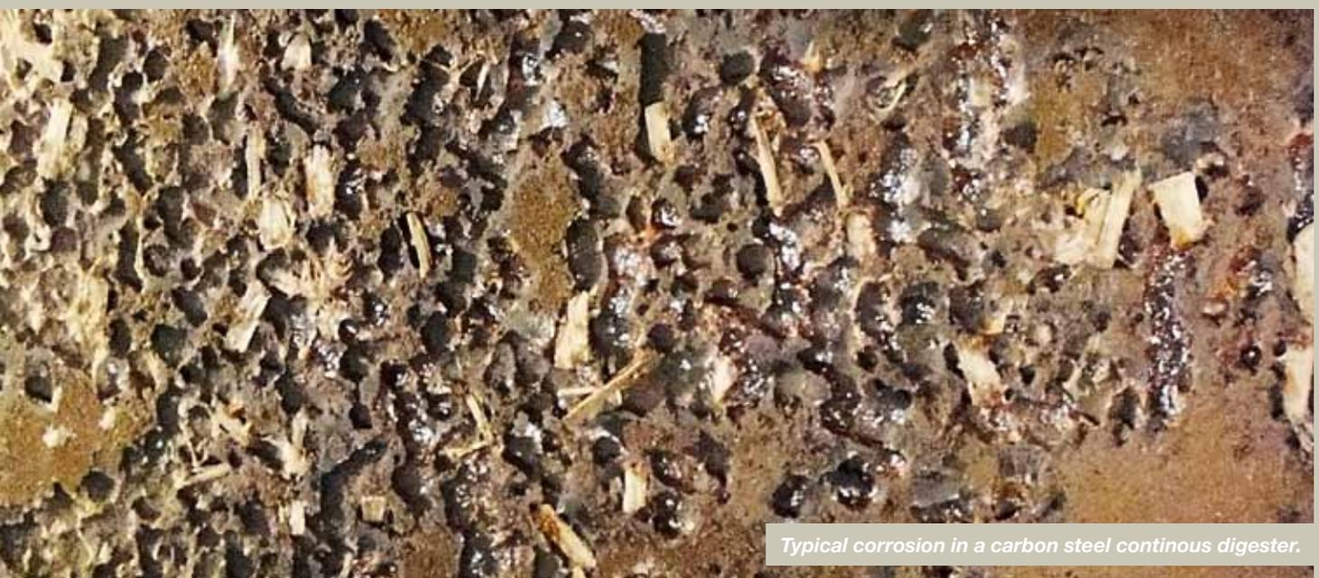
*Typical corrosion in a carbon steel continuous digester.*
