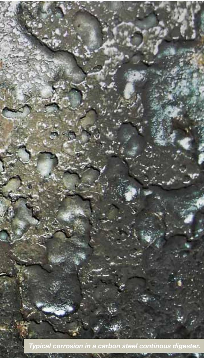
*Typical corrosion in a carbon steel continuous digester.*
